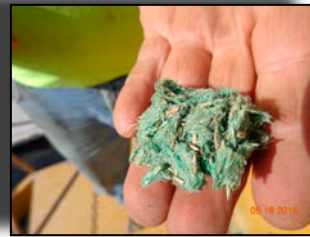
Hydroseeding mixture of grass seed and cellulose
